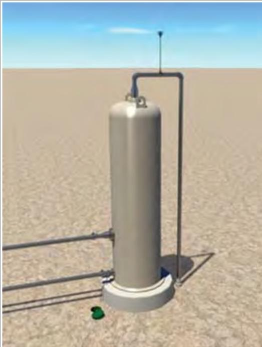
Dissipation Air Terminal above Process Tanks
