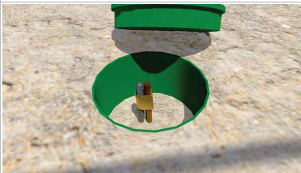
Class 1 Conductor Clamped to Ground Rod in
