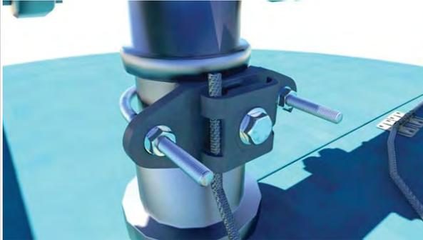
UL Rated Pipe Clamp Securing Class 1
