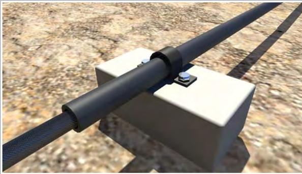
Class 1 Conductor Secured by Conduit
